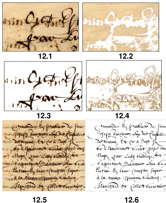
Figure 12. Results of the 3-means classification algorithm. 12.1. An extract of a degraded document image. 12.2. Image class n°1, 12.3. Image class n°2. 12.4. Image class n°3. 12.5. ancient manuscript with “bleed-through” interference provided by the archive of “Chatillon-Chalaronne” . 12.6. Restored image.
